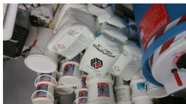
Sodium Bisulphate bags piled up and not protected from damage.
